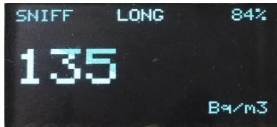
**Note:** The Sniffer must be running for more than 5 minutes for the 5-minute average to be accurate. But, once it has been running for 5 minutes, you can toggle between the short and long modes at any time, without waiting another 5 minutes.
